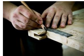
Measuring and marking out
