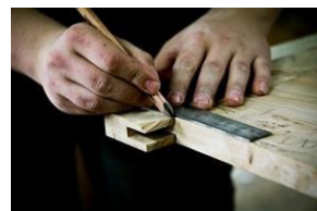
Measuring and marking out
